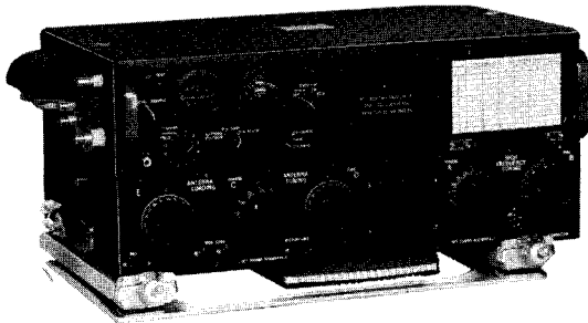
Figure 1-2. Type T-47/ART-13 Transmitter
