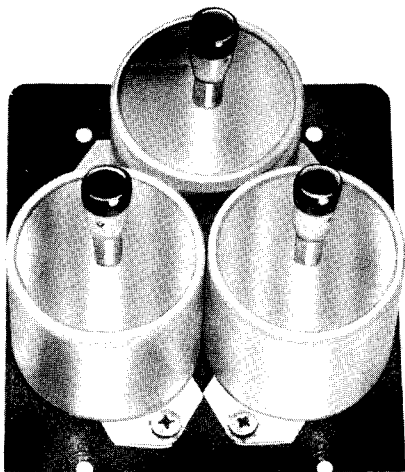
Figure 1-8. Type CU-24/ART-13 Antenna Shunt Capacitor
