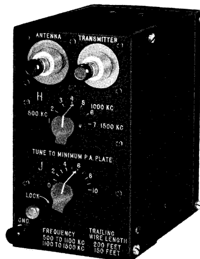
Figure 1-11. Type CU-26/ART-13 Antenna Loading Coil
