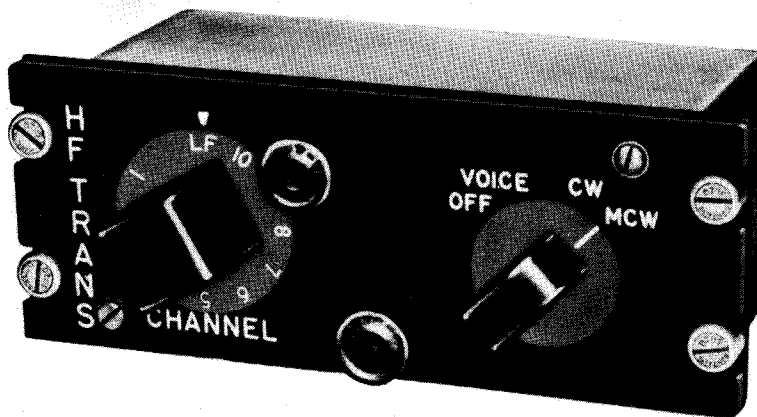
Figure 1-5A. Type C-740/ART-13 Pilot's Control Unit
